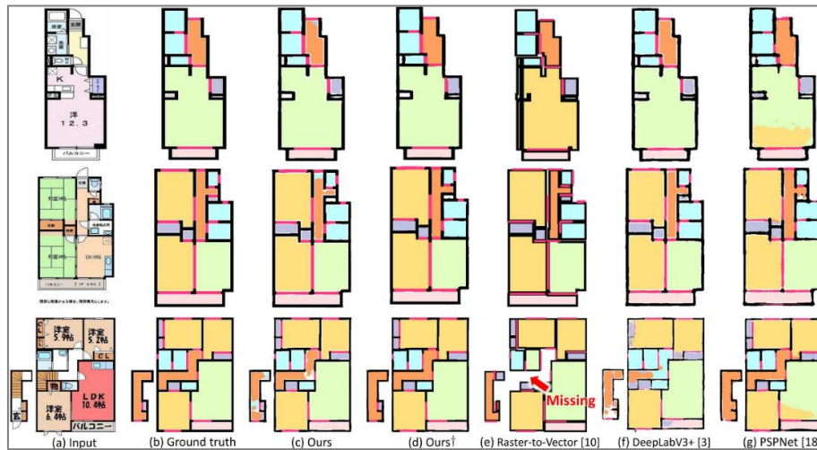
Figure 2.40. This study compares the segmentation results of all the algorithms given above (Zeng et al., 2019)
