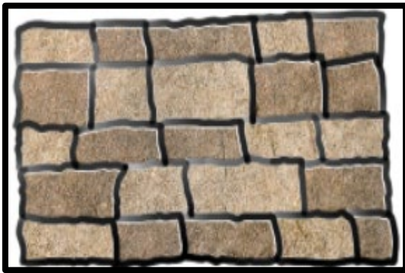
Figure 3.6. Coursed rubble masonry exterior view
