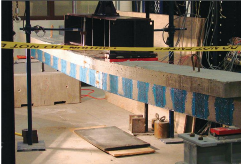
Figure 1.2. Concrete beam strengthened with CFR (Rasheed, 2015)
