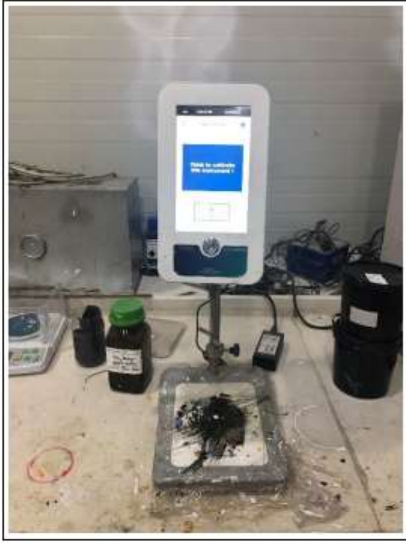
Resim 6.5. Lamy Rheology B-ONE PLUS Viskozimetre
