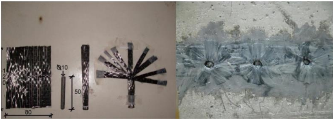
Figure 3.1. Fan type anchors used in the experimental program
