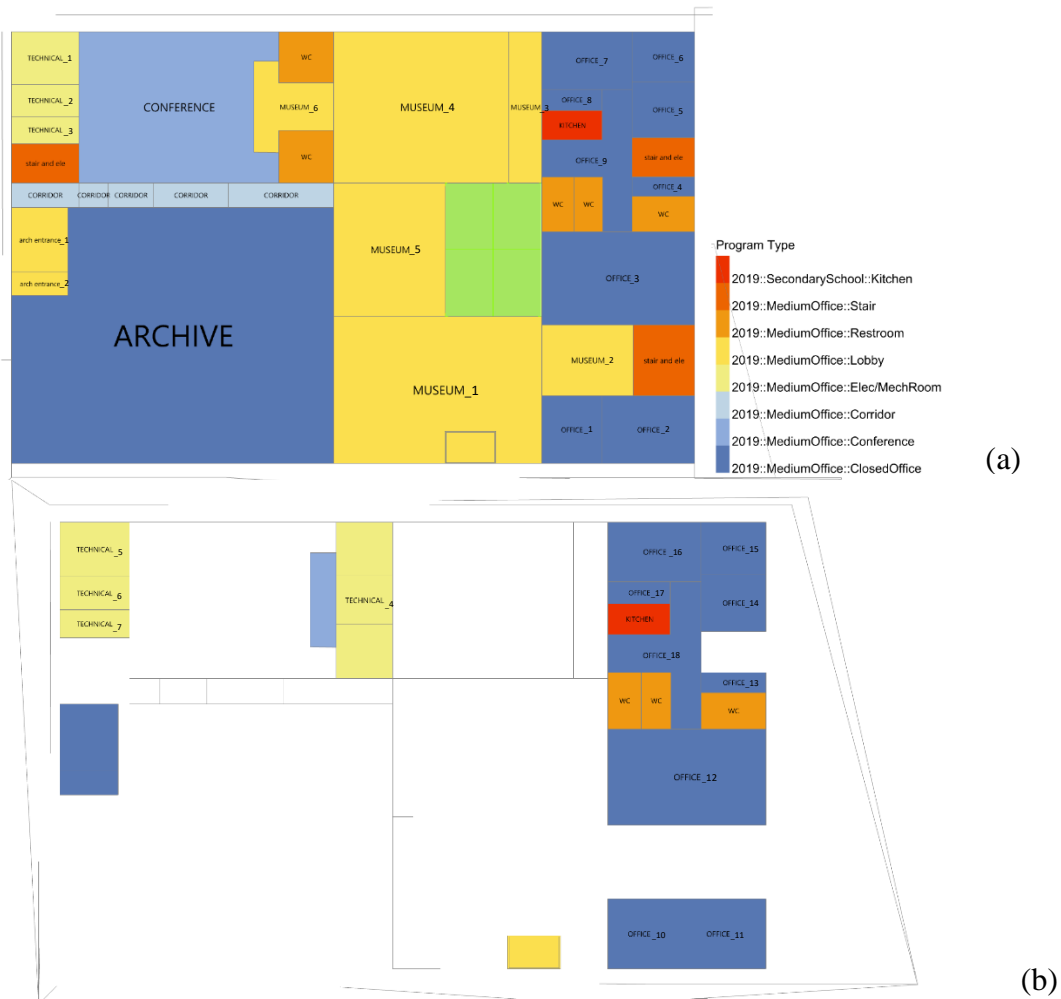
Figure 3.4. Thermal zones of the building a) ground floor plan b) first floor plan
