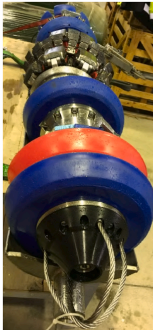
Fig. 11. MFL-PIG used during inspection.
