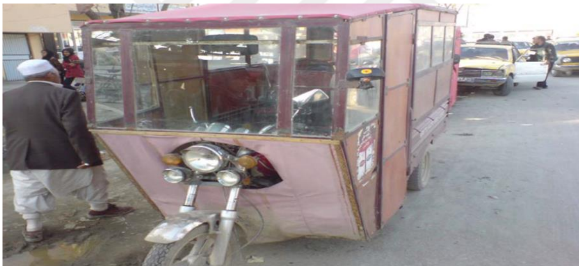
Figure 4.15. Shows the conversion of three-wheeled motorbikes into passenger-transporting autorickshaws. (Author, 15.10.2024)
