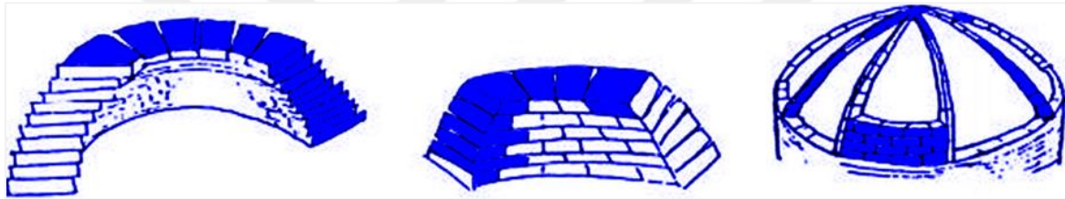
Figure 2.24. Three methods of the dome construction, adapted from (Ghasempourabadi, Mahmoudabadi Arani, Bahar, and Mahdavinejad, 2012).
