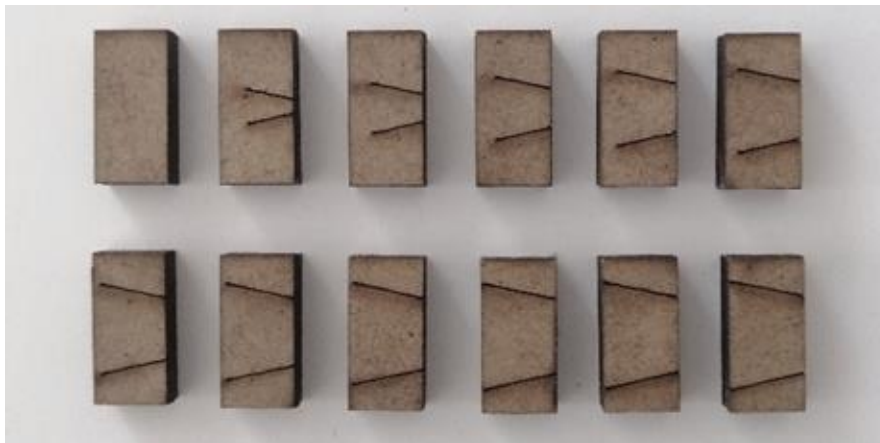
Figure 3.32. The corbel dome modal bricks and CNC laser scratched place marks on top.
