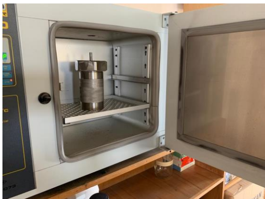
Image 4.2. Photograph of the mixture taken into a Teflon-steel autoclave
