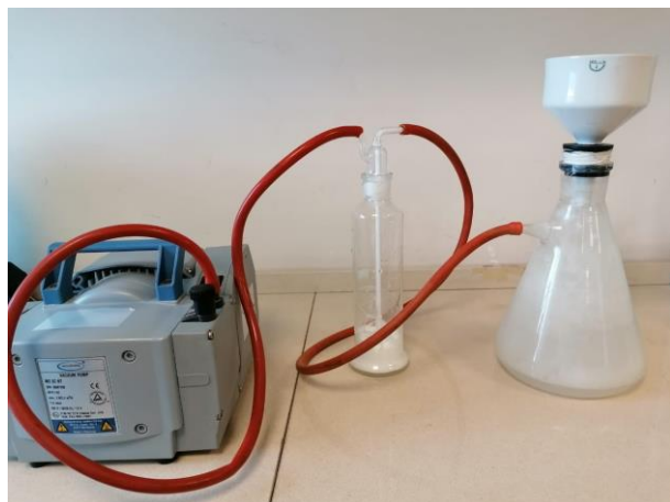
Image 4.4. Photograph of the washing process for the prepared sample
