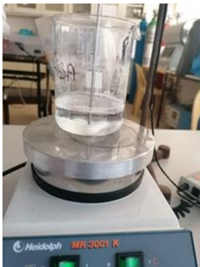
Image 4.8. Photograph of the surfactant's dissolving process in the deionized water at 30 °C using a magnetic stirrer
