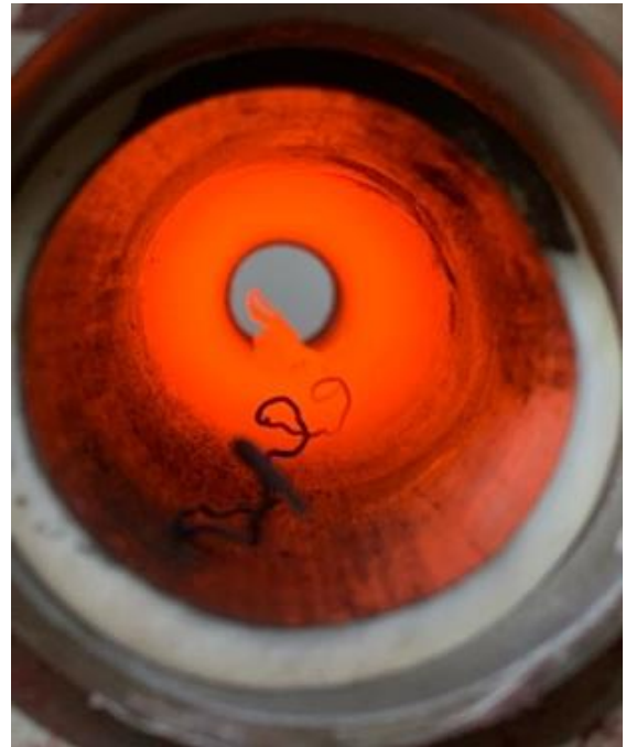
Figure 3. Austenitizing the specimen in a furnace
