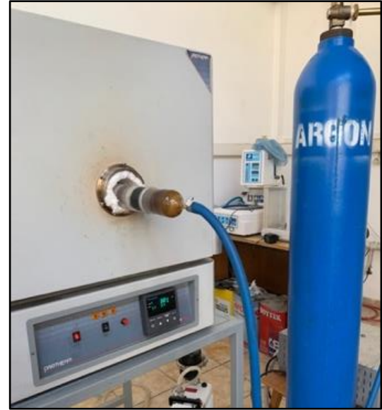
Figure 2. Protherm Furnace and Argon Gas Tube
