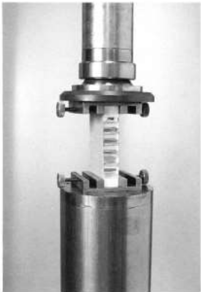
FIG. 1 Edge-wise Compression Test Setup
