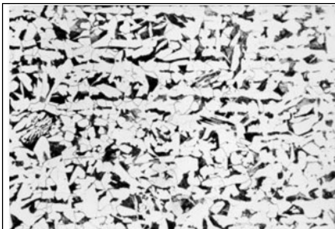
0.2% C steel Photo: J.Gibson
