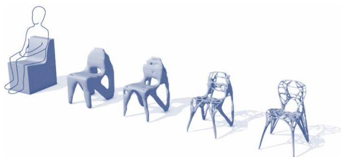
Figure 2.6. Topology optimization stages of a chair (Hemmerling & Nether, 2014).
