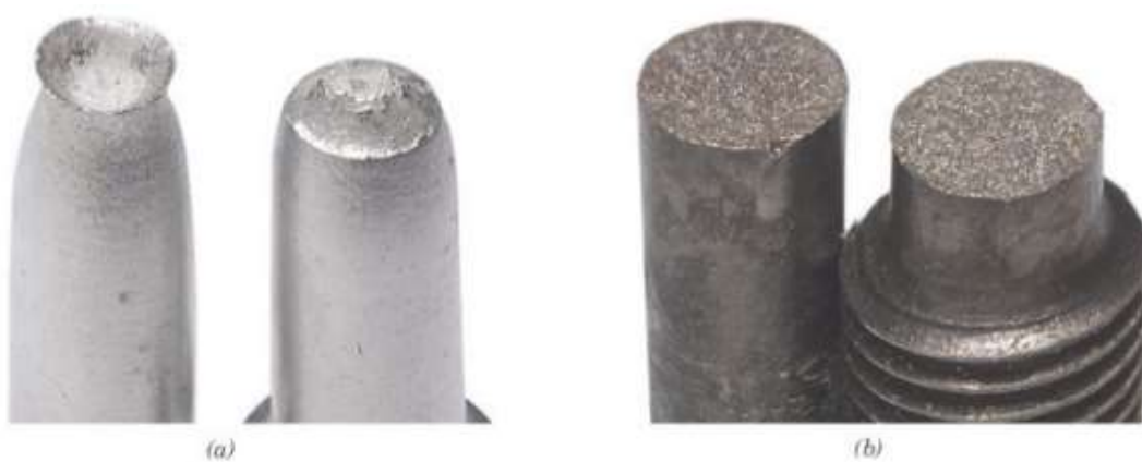
Fig 6. a) Ductile b) brittle fracture surface
