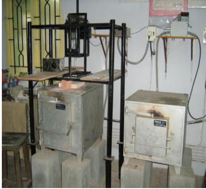
Figure 2. Schematic of the Stir Casting Setup and Furnace Assembly
