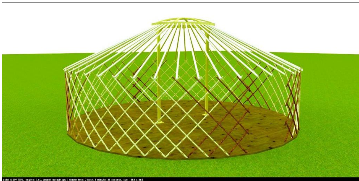
Figure 3.11. Structure of rafters
