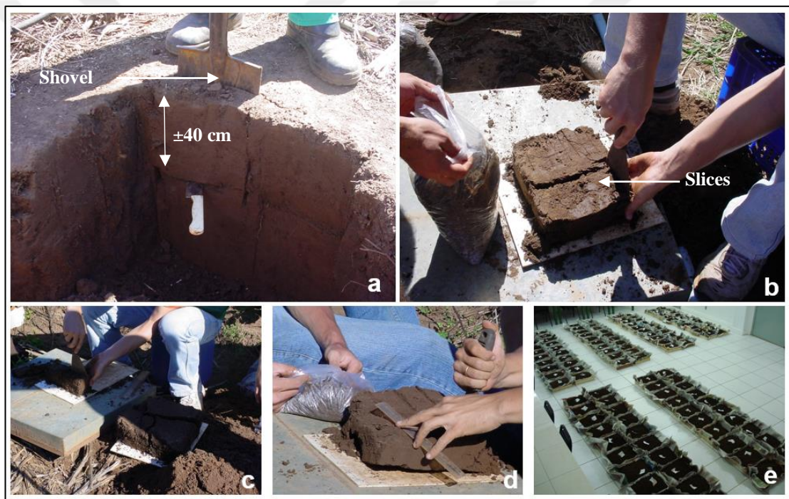
Figure 2.2. Sampling process a- Sampling with the help of a shovel b, c, and d- Layering process e- After sampling 1
