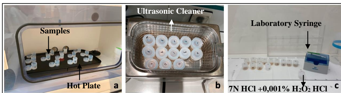
Figure 2.6. a- When samples were evaporated on the hot plate at 110°C b- Ultrasonic bath c- Adding 1.5 mL of 7N HCl +0,001% H 2 O 2 HCl to samples before chromatographic separation
