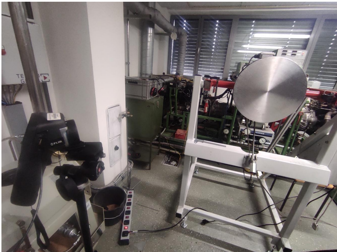
Figure 6.2. Heated rotating disk system with the thermal camera
