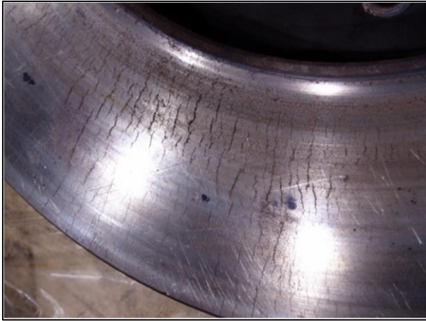
Figure 1.2. Thermal cracks in a railway brake disk [6]
