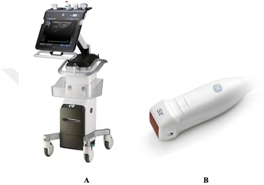
Şekil 9. A- GE Healthcare Venue Point of Care® USG cihazı, B- 4 MHz faz array kardiyak prob
