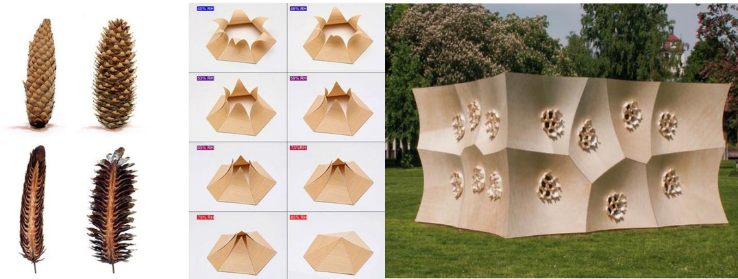
Figure 3.22. Scientific development: humidity responsive wood composites, photo of Hygroskin ( URL-14 )
